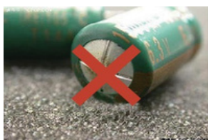
capacitor bulge and leakage
