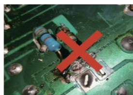
capacitor bulge and leakage
